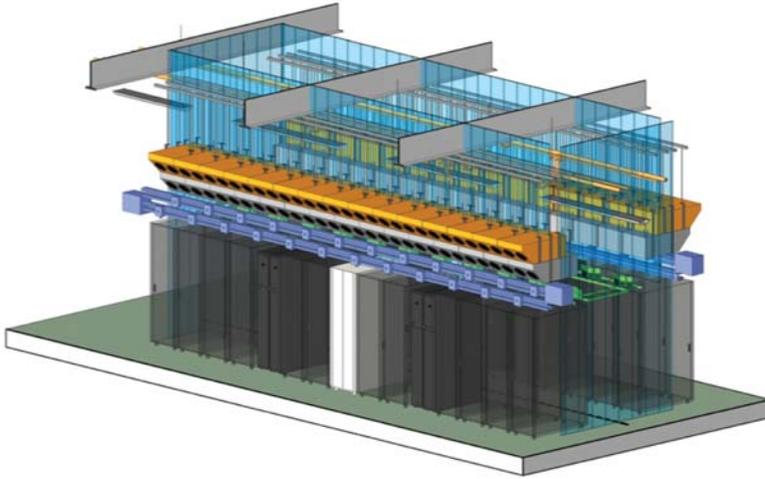
Figure 4. Oracle's pod design defines flexible, modular spaces that can be replicated in datacenters around the world. This design is for a Tier 4 datacenter with high-density equipment and a total capacity of 860 kW, or 45 kW per rack.
