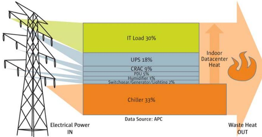
Figure 1. Only a fraction of incoming power is delivered to the IT equipment in a datacenter, underscoring the need for both server and infrastructure efficiency improvements.
