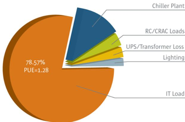
Figure 3. Oracle's Santa Clara, California, datacenter achieved a percent of its power budget is delivered to IT equipment.
